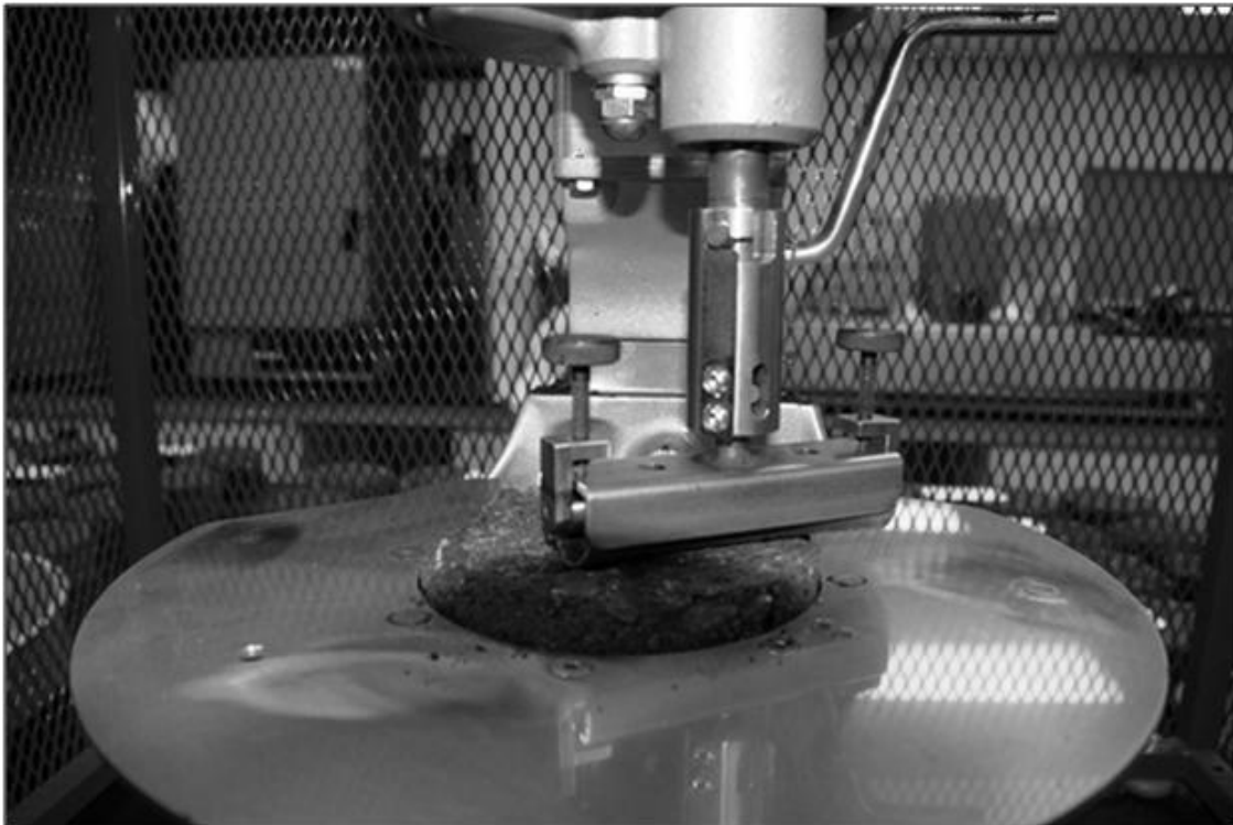
Figure 4. Close-up of Ravelling Test in Progress
